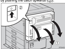
Open the right cover by pushing the catch upwards.
