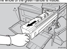
There is the green lever (1) on the left side of the fusing unit. While pressing the green lever to the left, slide the fusing unit out slowly with rasing the green handle and
