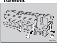
Align the new development unit with the rail in the printer. Slide the development unit into the printer until it makes a click as it locks into place.
