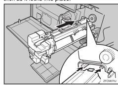
At the right side of the printer, remove the tape on the left and right sides of the black sheet, and then pull out the sheet using both hands.
