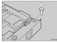
Remove the screw inside the front cover (1) by turning it counterclockwise to release the fusing unit.
