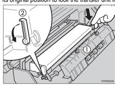
☐ If you cannot return the green lever to its original position, raise the green lever and remove the transfer unit. After that, try to install the transfer unit again.
