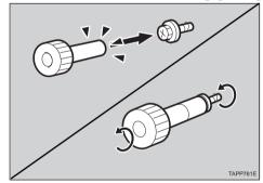
☐ You need the screw to lock the new fusing unit afterwards.
