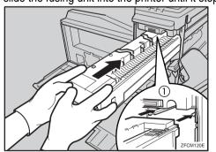
Lock the fusing unit in place with the screw you removed in step 3.
