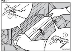
While pressing down on the corner of the transfer unit indicated by the arrow (①), return the green lever (②) to its original position to lock the transfer unit in place.
